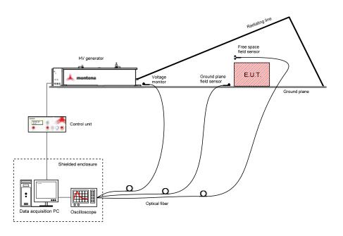
Montena systems include a range of standard size installations for EUT from a height of 50 cm up to large structures such as vehicles or airplanes. The smallest systems are transportable and can be set up and removed in less than 2 hours.
