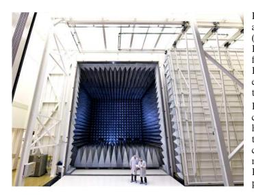
ETS-Lindgren installed a large RF shielded anechoic chamber for Passive Intermodulation (PIM) emissions testing of satellites at the Lockheed Martin Company (LMCO) production facility in Sunnyvale, California. Certifying that a LMCO satellite is not producing PIM emissions expedites development schedules, allowing LMCO to better meet commitments to its customers.
