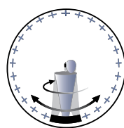
Multi-Antenna Distributed-Axis Scanning Method Shown with Optional Goniometer
